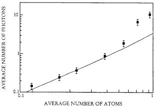
NUMBER OF PHOTONS at equilibrium versus the number of atoms in the high-Q cavity of a single-atom laser as an atomic beam passes through. Photons leaking from the mirrored ends of the cavity constitute the laser beam. Solid curve is the prediction of a one-atom quantized field model. (Adapted from ref. 1.)
